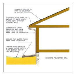
Gutters and downspouts should be kept free of leaves and other debris for optimal function. Gutter downspouts should discharge water at least five feet from the foundation and past any landscape edging. Do not remove these extensions since they provide a path for the roof water to flow away from the backfill soils and foundation.
