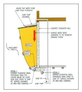
you should install one. Otherwise, it is possible the water in the pit will rise and flood your crawl space or basement. Remove debris or sediment at the bottom of the pit using a wet shop vacuum so that the inlet pipe does not become clogged. Periodically pour water into the sump pit to check the operation of the pump's float control. If the float control is broken, the pump will not turn on when the water level rises, which could lead to flooding of your basement or crawl space.
