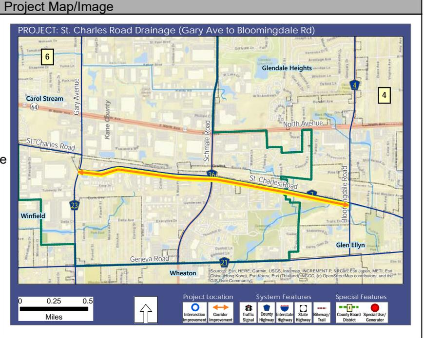
**Description** Reconstruct poor drainage systems along St. Charles Road. Project includes replacement of culverts, regrading ditches, improving stormwater flow to and from creeks and wetlands. Environmental engineering and design engineering to be completed through various contracts.
