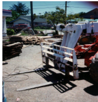
A winch was welded on the boom of this telescoping truck without prior manufacturer’s approval.
