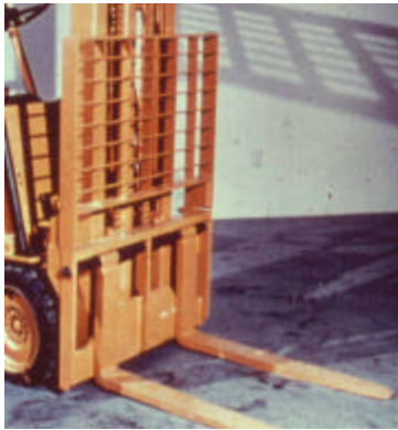
A backrest extension keeps the load from falling rearward.
