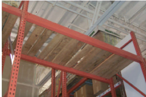
Check that wood stringers or decking in racks are in good condition. They may support the load if the pallet is not properly placed on both front and rear rails.
