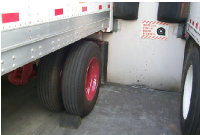
Chock the rear wheel of trucks and trailers to prevent movement away from the dock. Notice the sign tells drivers to chock the wheels.
