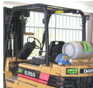
An overhead guard can deflect objects falling from above.
