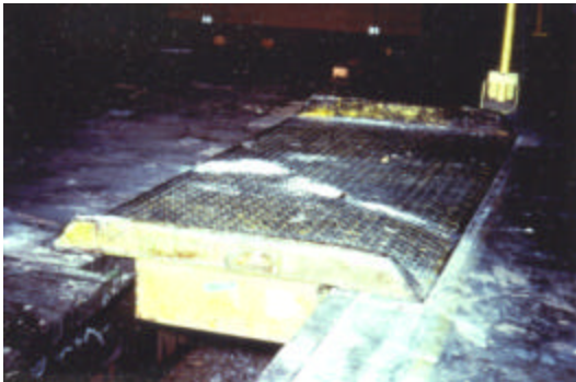
A projection below the surface prevents the dock board from shifting off its support.
