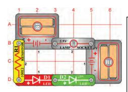
In this circuit the LED's (D1 & D2) will have the same brightness, but the lamp (L1) will be off. When connected in series, all components will have equal electric current through them. The lamp is off because it requires a higher current through the circuit to turn on than the LED's do.
