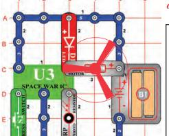
This circuit is activated by light on the photoresistor, (RP) though the fan will barely turn at all. Press the press switch (S2) and the fan will spin. If you hold the press switch down, the fan will spin faster. If you cover the photoresistor, the fan will stop unless the press switch is pressed.
