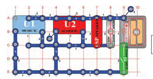
In the circuit, the outputs from the alarm (U2) and music (U1) IC's are connected together. The sounds from both IC's are played at the same time.
