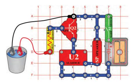
OBJECTIVE: To sound an alarm when water is detected.
