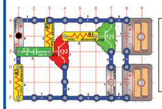
Install the parts. The lamp (L2) will be on. It will be off as long as you blow on the mic (X1). Speaking loud into the mic will change the brightness of the lamp.
