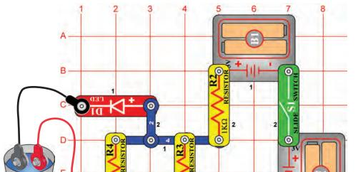
OBJECTIVE: To show how water conducts electricity.
