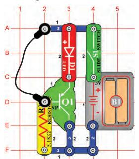
OBJECTIVE: To build a transistor light alarm.
