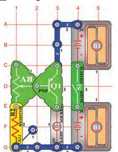
**OBJECTIVE:** To demonstrate adjusting the gain of a transistor circuit.
