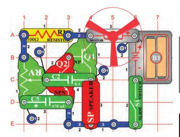
Build the circuit on the left and place the fan onto the motor (M1). Turn on the slide switch (S1) and move the setting on the adjustable resistor (RV) across its range. You hear screaming sounds and the fan spins.
