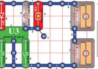
Build the circuit shown on the left. Activate the circuit by turning on the slide switch (S1) or pressing the press switch (S2), do both several times and in combination. You will hear exciting sounds and see flashing lights, as if a space battle is raging!
