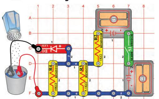
OBJECTIVE: To show how adding salt to water changes water's electrical characteristics.
