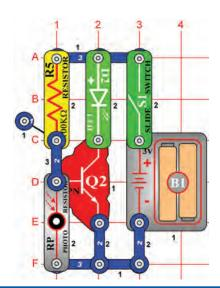
OBJECTIVE: To compare transistor circuits.
