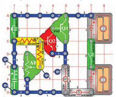
OBJECTIVE: To build a lamp that stays on for a while.
