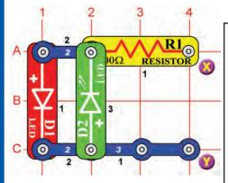
Use this circuit to check the polarity of a battery. Connect your battery to X & Y on the drawing using the jumper cables (your 3V battery pack (B1) can also be snapped on directly instead). If the positive (+) side of your battery is connected to X, then the red LED (D1) will be on, if the negative (-) side is connected to X then the green LED (D2) will be on.
