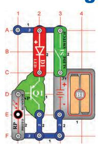
OBJECTIVE: To compare transistor circuits.
