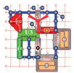
OBJECTIVE: To build a fan with sound that is activated by light.
