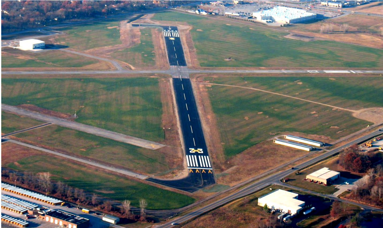
Figure 2-3. Markings for a Temporarily Closed Runway
