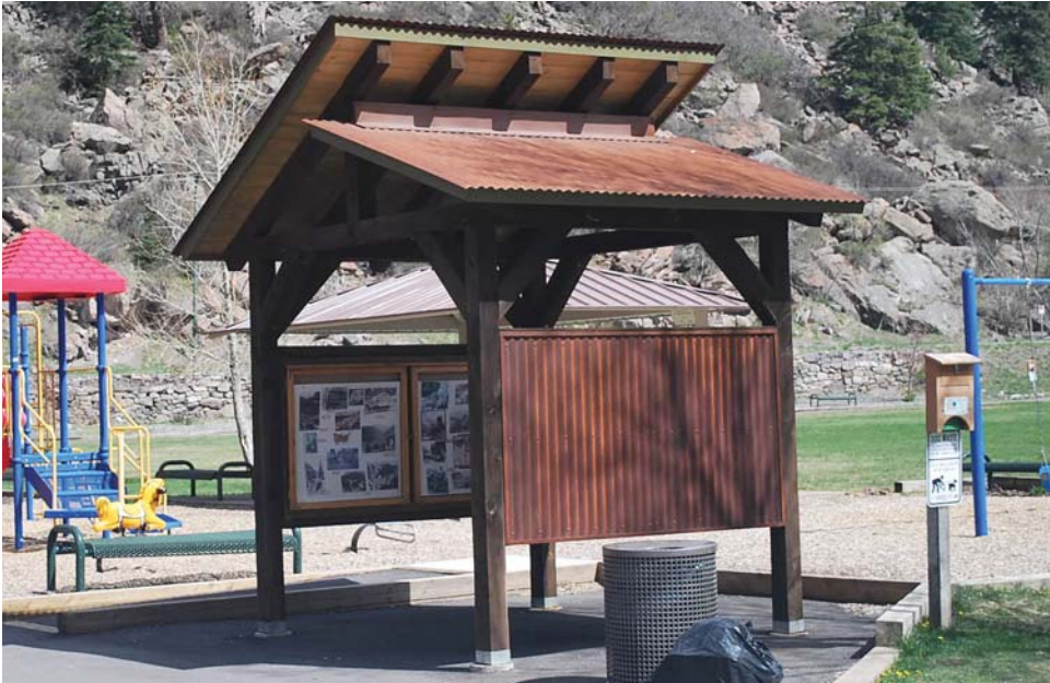
Fellin Park Kiosk (Materials Precedent) This existing kiosk found in Fellin Park features the desired materials to be utilized in both the proposed new stage and restroom facilities. Corrugated weathering steel roofing and siding with wooden beams are featured in this structure.
