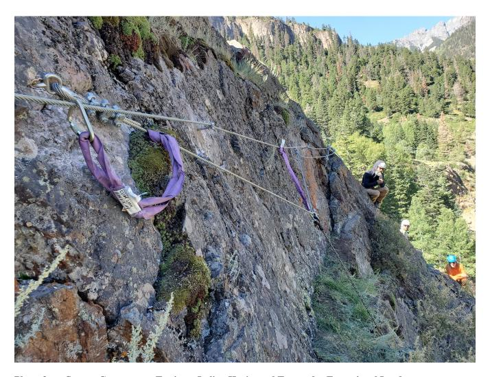
Photo 3: System Components Testing – Italian Horizontal Test under Exceptional Load
