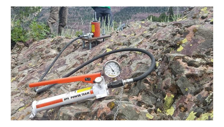
Photo 1: Bolt Pullout Testing - Hydraulic Pump and Hollow Ram Apparatus
