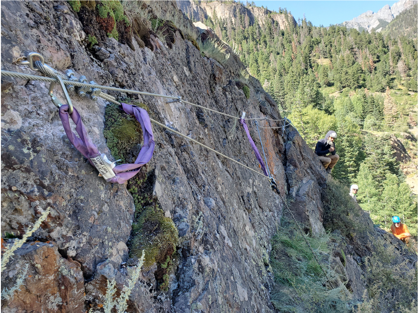
Photo 3: System Components Testing – Italian Horizontal Test under Exceptional Load
