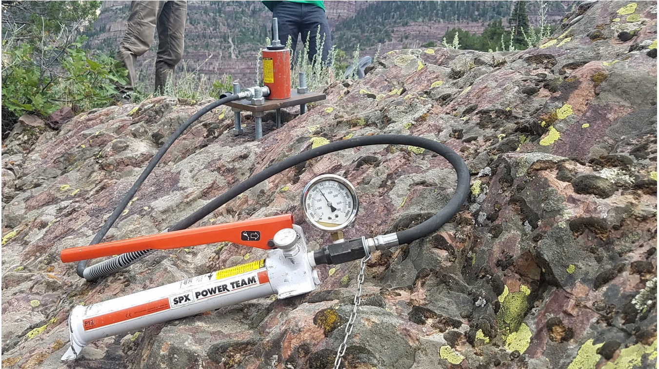
Photo 1: Bolt Pullout Testing - Hydraulic Pump and Hollow Ram Apparatus
