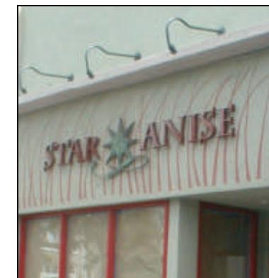
**WALL SIGNS** ARE TO BE MOUNTED FLUSH AND FIXED SECURELY TO A BUILDING WALL, PROJECTING NO MORE THAN 30 INCHES FROM THE FACE OF A BUILDING WALL, AND NOT EXTENDING SIDEWAYS BEYOND THE BUILDING FACE OR ABOVE THE WINDOW SILL OF THE SECOND STORY WINDOW.
