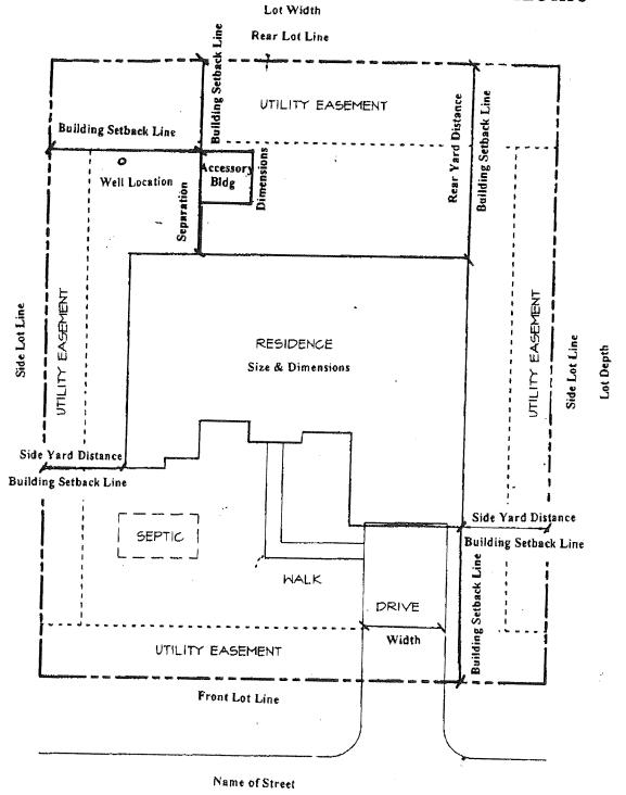
Showing all existing and proposed structures sizes/locations, property lines, Right-of-ways, Driveways, Water bodies, well/Septic locations easements, LP Gas Tanks etc...
