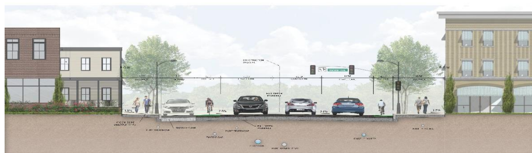
PROPOSED SECTION WITH TURNING LANE AT INTERSECTION
