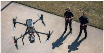
Drone equipped with Forward Looking Infrared (FLIR) system. The drone is used during special events, search and rescue, and tactical deployment on active crime scenes.
