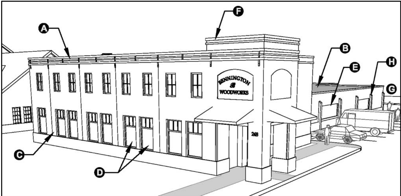
Figure G2.1: Breaking Up the Masses Helps Reduce the Scale. Dividing the building volume up into a variety of shapes helps to reduce the perceived scale of the architecture and allows placement of the more important volumes up near the front of the site.
