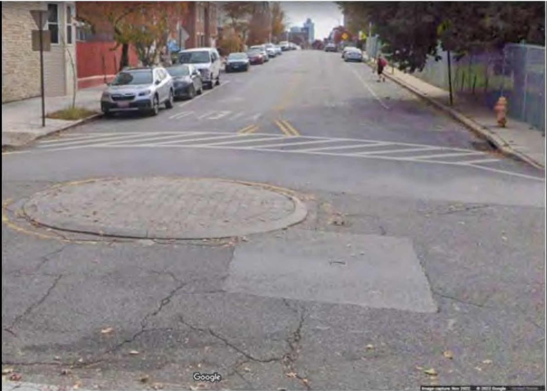
Figure 41. Example Traffic Calming Roundabout.
