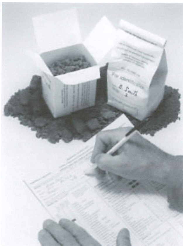
Figure 5. Thoroughly mix the air-dried sample, fill the sample bag or box, mark with your sample designation, fill out the information sheet, and take the sample to your county Extension office.
