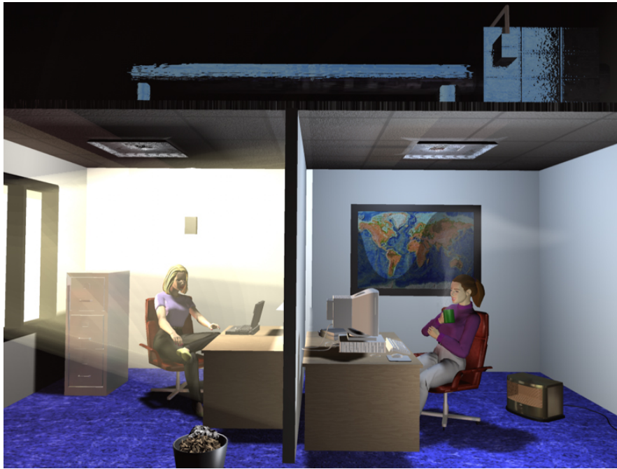
Figure 2 Central air handling system serving two rooms illustrating dissimilar heating/cooling requirements due to solar heat gain through windows.
