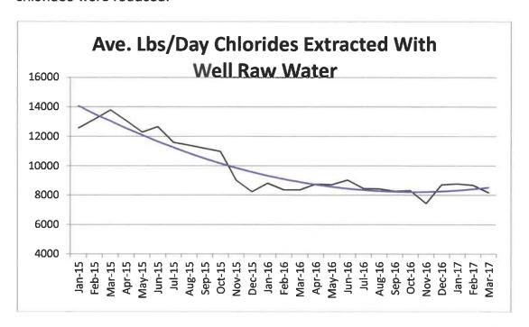
This is turn has a direct correlation with the pounds of chlorides discharged with the WWTP effluent.
