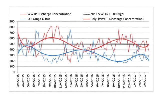
The chart below is a plot of the effluent flow in relation to the effluent concentration. Note that as we approach the 3 MGD flow most of the test points fall below the 500 limit with none going above 600 mg/l. The linear interpretation of the data points indicates that for each MGD of flow the chloride concentration will drop about 70 mg/l.
