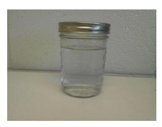
After running for about 20 hours the water cleared up very well and the chlorides stabilized at about 320 ppm. This is a great quality raw water, however, capacity is now the issue. We must do further testing with a larger test pump to determine if the well production will sastifactory.
