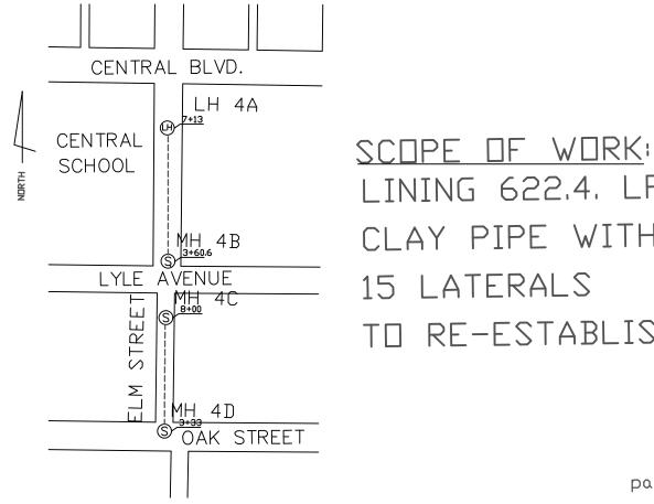
\_INING 622,4, LF OF 8" CLAY PIPE WITH 15 LATERALS TO RE-ESTABLISH.
