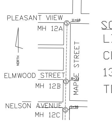
SCOPE OF WORK: LINING 570 LF OF 12" CLAY PIPE WITH 13 LATERALS TO RE-ESTABLISH.
