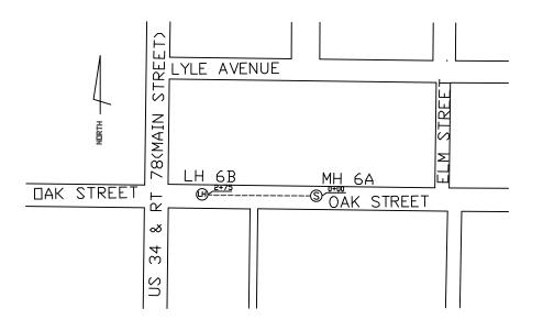
SCOPE OF WORK: LINING 275 LF OF 8" CLAY PIPE WITH 5 LATERALS TO RE-ESTABLISH.
