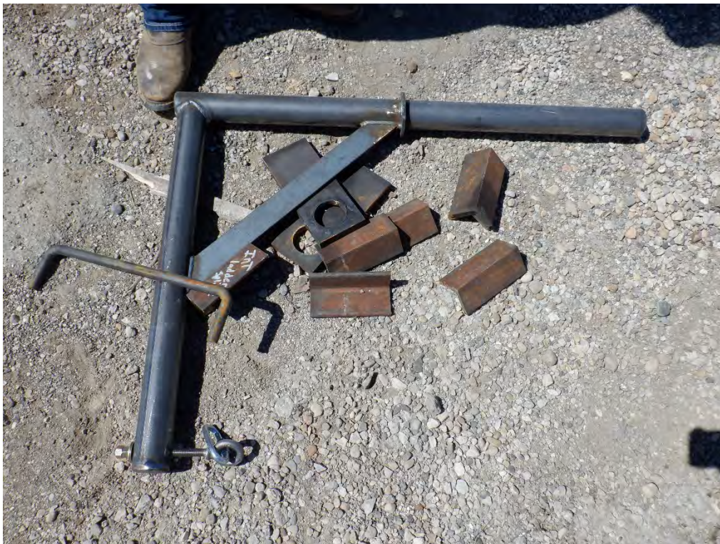
PHOTO #2: Purposed davit arm. Waiting for stamped drawings by an IL structural engineer before approval can be given to use this design.
