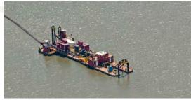
Design Dredge Contract for the State of Kansas Water Office to remove sediment from a federally owned reservoir. Contract included design and construction of confined placement areas, over 30,000 lf of dredge discharge pipeline, and 6,000 lf of effluent discharge pipeline. Dredging started May 2016 and was completed in October 2016. *Quantity:* 3 million cubic yards
