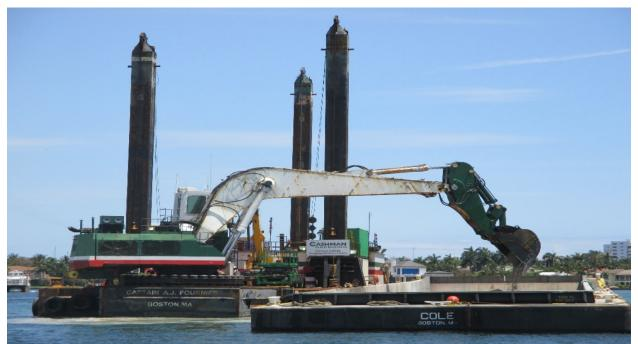
Photograph 3.1 Mechanical Dredge and Hopper Barge in the ICWW, Broward County
