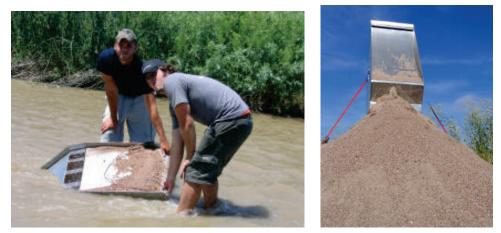
Figure 6. 2 ft collector and drop box used to estimate production rates.
