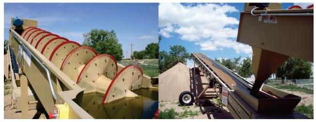
Figure 3. Archimedes screw separator (left) and stacker (right).
