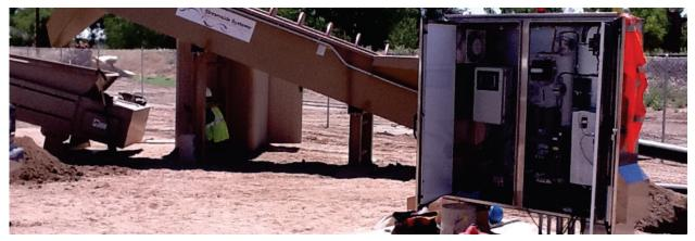
Figure 4. Electronic control panel and Archimedes screw separator.
