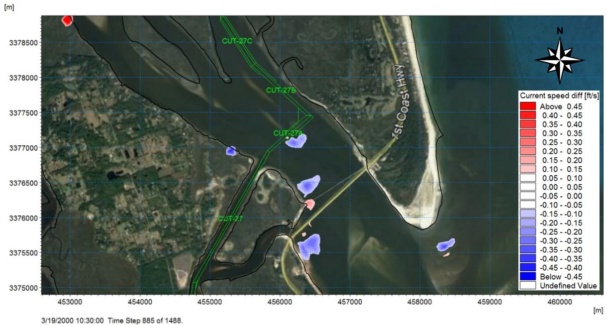
**Figure 4.16** Difference in Modeled Alternative C and Baseline Peak Ebb Velocities
