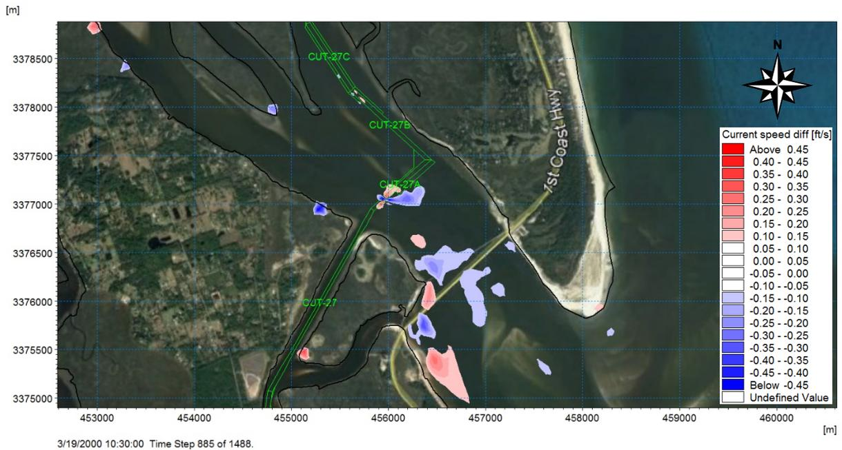
**Figure 4.14** Difference in Modeled Alternative B and Baseline Peak Ebb Velocities
