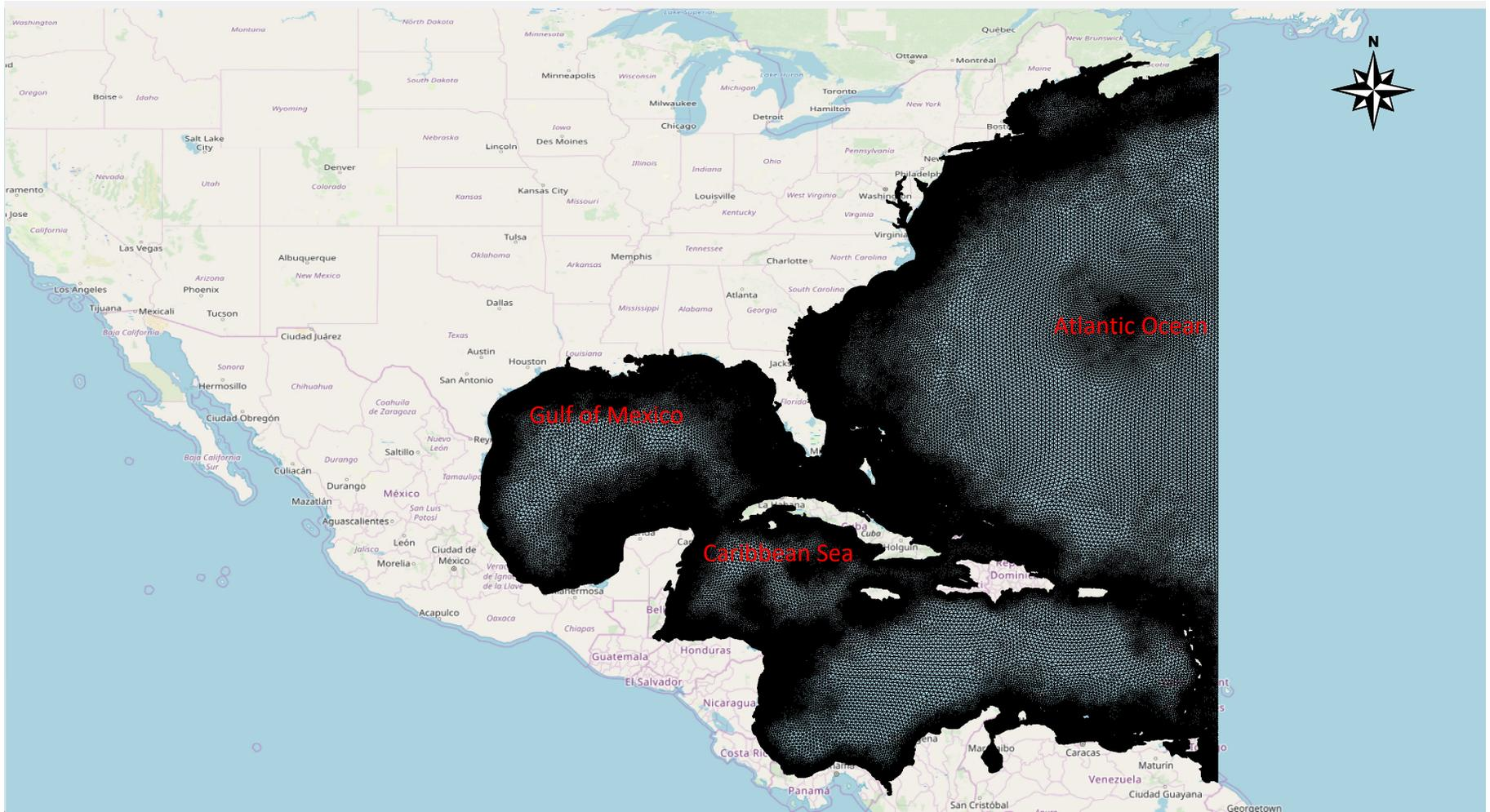
Figure 2.9 FEMA Northeast Florida-Georgia Version 12b ADCIRC Model Mesh
