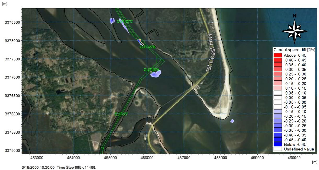
**Figure 4.22** Difference in Modeled Alternative F and Baseline Peak Ebb Velocities
