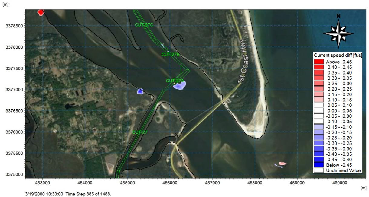
**Figure 4.12** Difference in Modeled Alternative A and Baseline Peak Ebb Velocities
