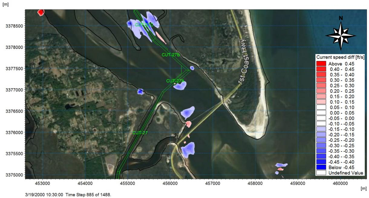
**Figure 4.18** Difference in Modeled Alternative D and Baseline Peak Ebb Velocities
