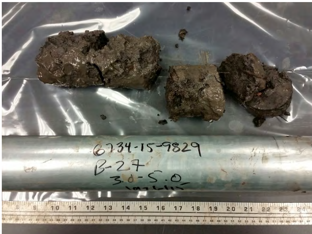
Photo 19: Thin-walled tube sample from Boring B-27, depth range of 3.0 to 5.0 ft.
