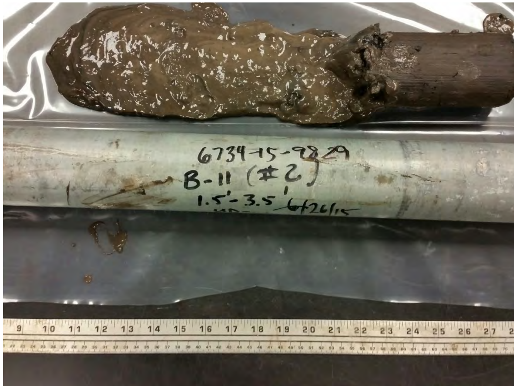
Photo 18: Thin-walled tube sample from Boring B-11, depth range of 1.5 to 3.5 ft.
