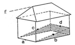
a, b, c, d = avg finisthed grade on each building wall Average Grade (entire building): (a+b+c+d)/4 = e Height = f (elevation at peak) – e (average grade)
